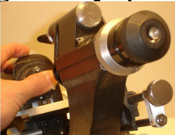
With the Lensometer in the Off position, cover the lens stop
