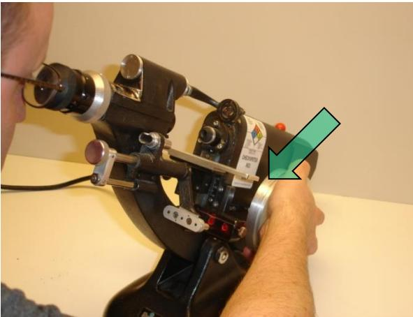
While looking into lensometer, turn power drum topside-towards-you until lines are clear
